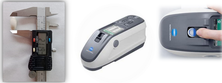
Figure 8 Caliper and colorimeter used to obtain morphological and colour data of faba beans in all formats.
